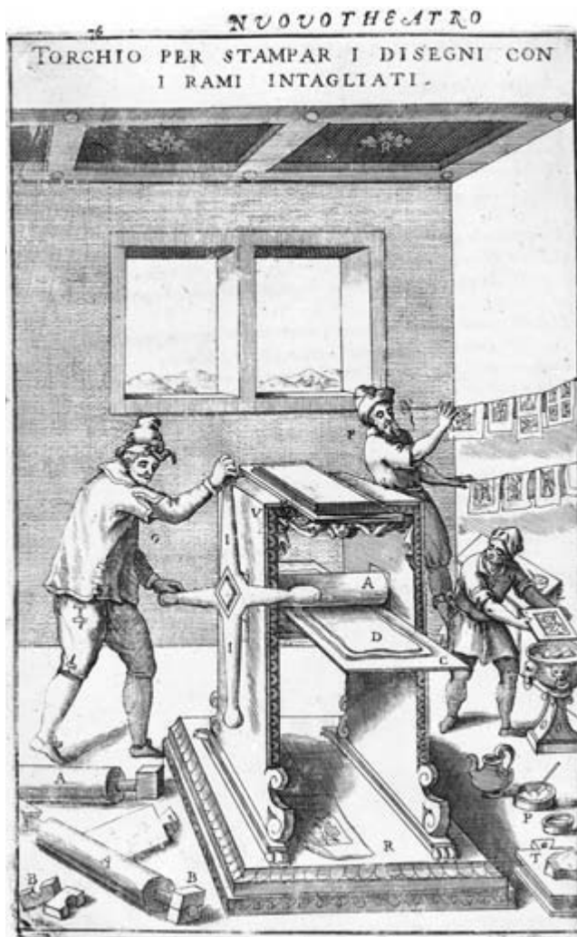
FIG. 22.9. INTAGLIO ROLLING PRESS. The rolling press relied on a different action than the letterpress screw press, providing intense pressure on plate and paper as they were passed through the rollers. Note the apprentice heating the copperplate before inking it.
