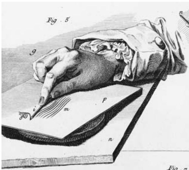
FIG. 22.6. HOLDING THE GRAVER. The tool required very little pressure, being held between the thumb and forefinger. Size of the detail: ca. 10.5 × 12.1 cm. Denis Diderot and Jean Le Rond d'Alembert, Encyclopédie (Paris: Briasson, 1751), tome 5, pl. III (section headed "Gravure"). Photograph courtesy of the BL (Rar 034.1, Plates, Tome 5).
